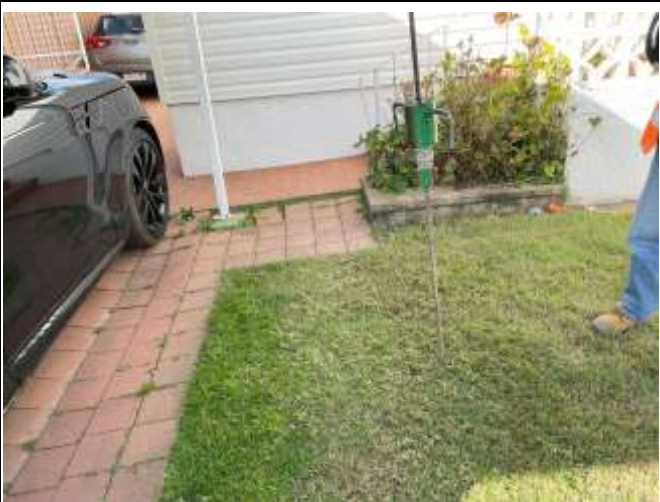
Photograph 2 DCP test in progress at location of DCP2 within front yard
