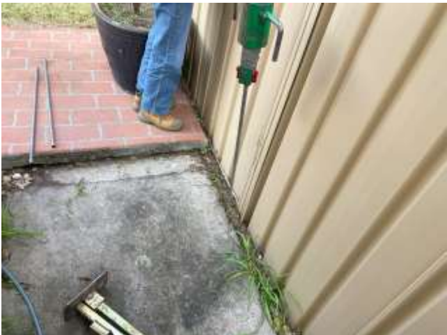
Photograph 3 DCP test in progress at location of DCP3 within rear portion
